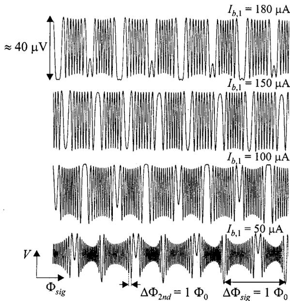
FIG. 3. Experimental  $V-\Phi_{\text{sig}}$  characteristics of the two-stage SQUID system with DROS A as the second stage for different bias currents of the first stage, indicated at the right. The signal flux was applied via the feedback coil of the first stage. The bias current of the second stage was fixed at  $I_{b,2} \approx 54 \mu\text{A}$ .
