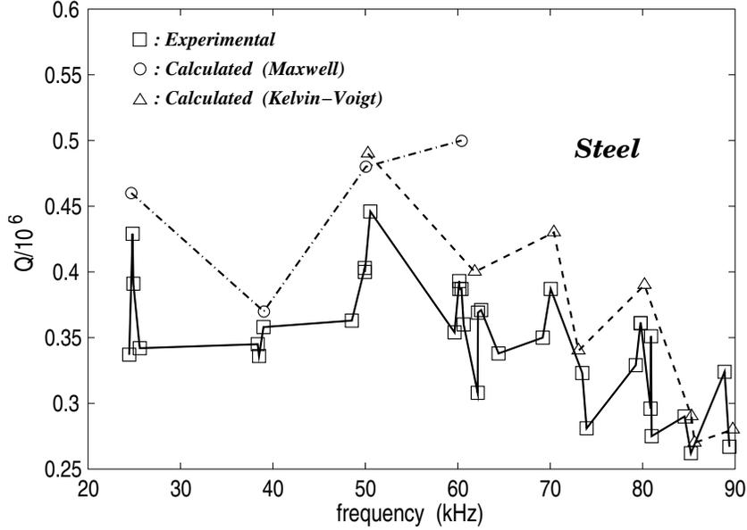
**Figure 3.** Quality factors of a sample sphere of steel; the sample had a diameter of 107 mm and measurements were taken at a temperature of 4 K. Lower frequency  $Q$ 's are fairly well fit by a Maxwell model with a viscoelastic ratio  $h' = 0.3$ , while higher frequency  $Q$ 's require a Kelvin-Voigt with viscoelastic ratio  $h' = 2.5$ . In this case there are more experimental points than theoretical due to mode splitting caused by the sphere suspension —see text.
