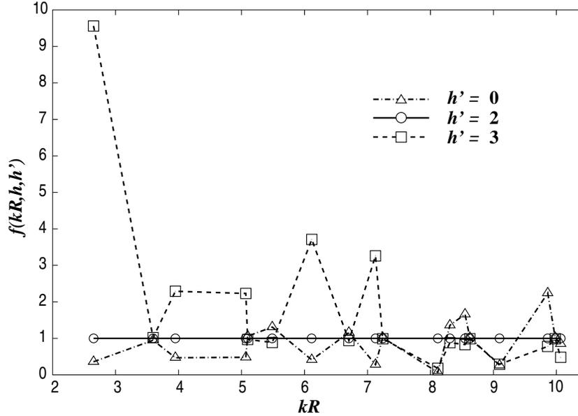
**Figure 1.** Plot of the function  $f(kR, h, h')$  —see (34)— for a Poisson ratio  $\sigma = 1/3$  (which means  $h = 2$ ), and for the first 18 (spheroidal) modes of the sphere's spectrum and a few values of the viscoelastic ratio  $h'$ . Note that  $f(kR, h, h') \equiv 1$  if  $h = h'$ .
