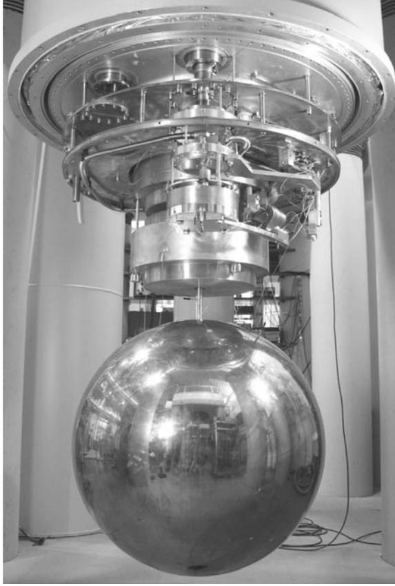
Figure 1. The ultracryogenic antenna MiniGRAIL.
