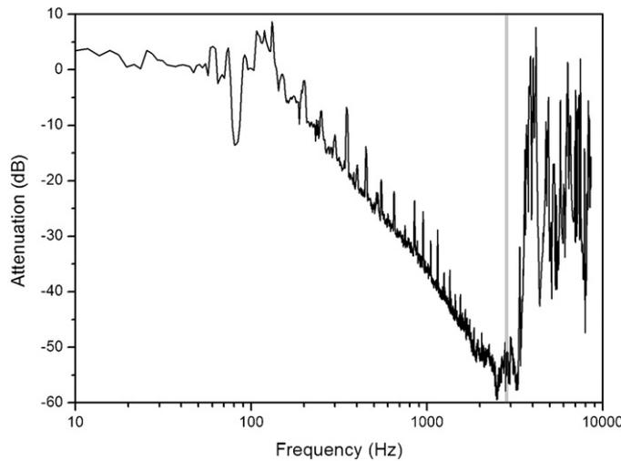
**Figure 1.** The attenuation between masses 3 and 4 of the vibration isolation system after modification. The grey area indicates the frequency range of the five spheroidal quadrupole modes of the bare sphere. All measurements were done at room temperature in air.
