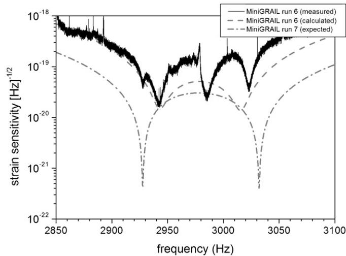
**Figure 2.** The spectral strain sensitivity of MiniGRAIL as achieved in run 6 at a temperature of 5 K compared to the simulation of a simple two-mode system. The expected sensitivity curve of MiniGRAIL when operated at a temperature of 80 mK is also plotted.
