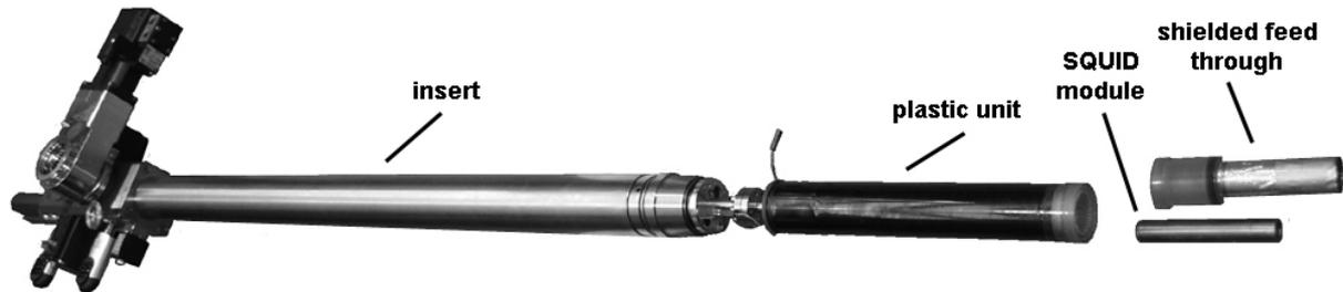
**Figure 5.** Picture of the ultra-cryogenic SQUID test facility using a MCK-50-100 commercial plastic dilution refrigerator. The fridge was modified with a special shielded feed through to the mixing chamber, so that the SQUID module can be directly inserted in to the liquid.
