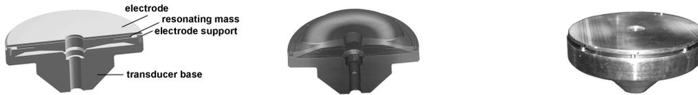
**Figure 3.** 3D model, simulation and prototype of the advanced transducer.
