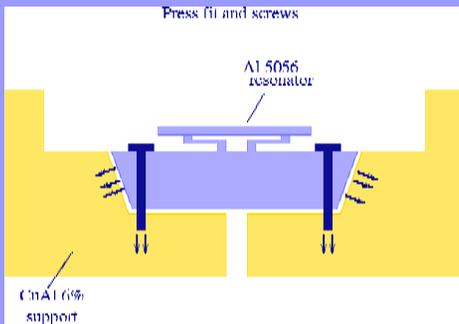
resonator press fit in a
